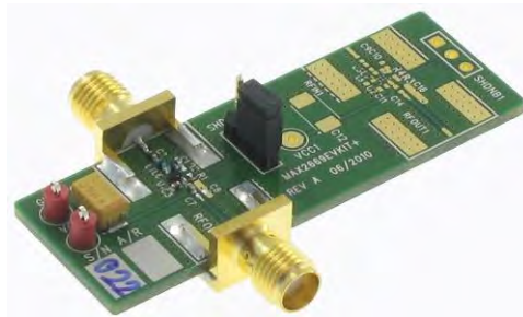
Figure 10. Maximum Integrated MAX2669 LNA Kit (Figure provided by [7])
