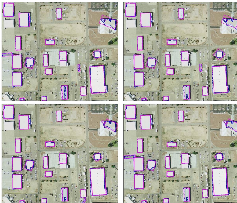
Figure 4.4: Sample variations in the result of the building extraction algorithm applied to Image 2. Original image data available from the U.S. Geological Survey [1].
