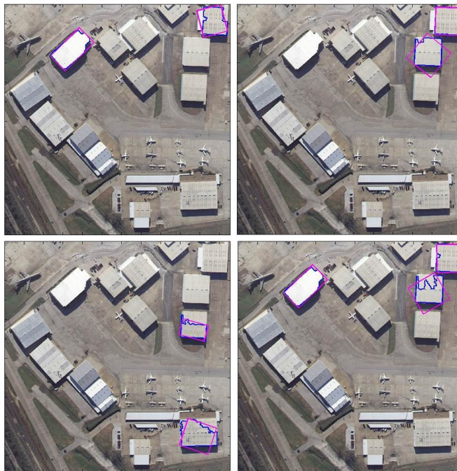
Figure 4.10: Sample variations in the result of the building extraction algorithm applied to Image 5. Original image data available from the U.S. Geological Survey [1].
