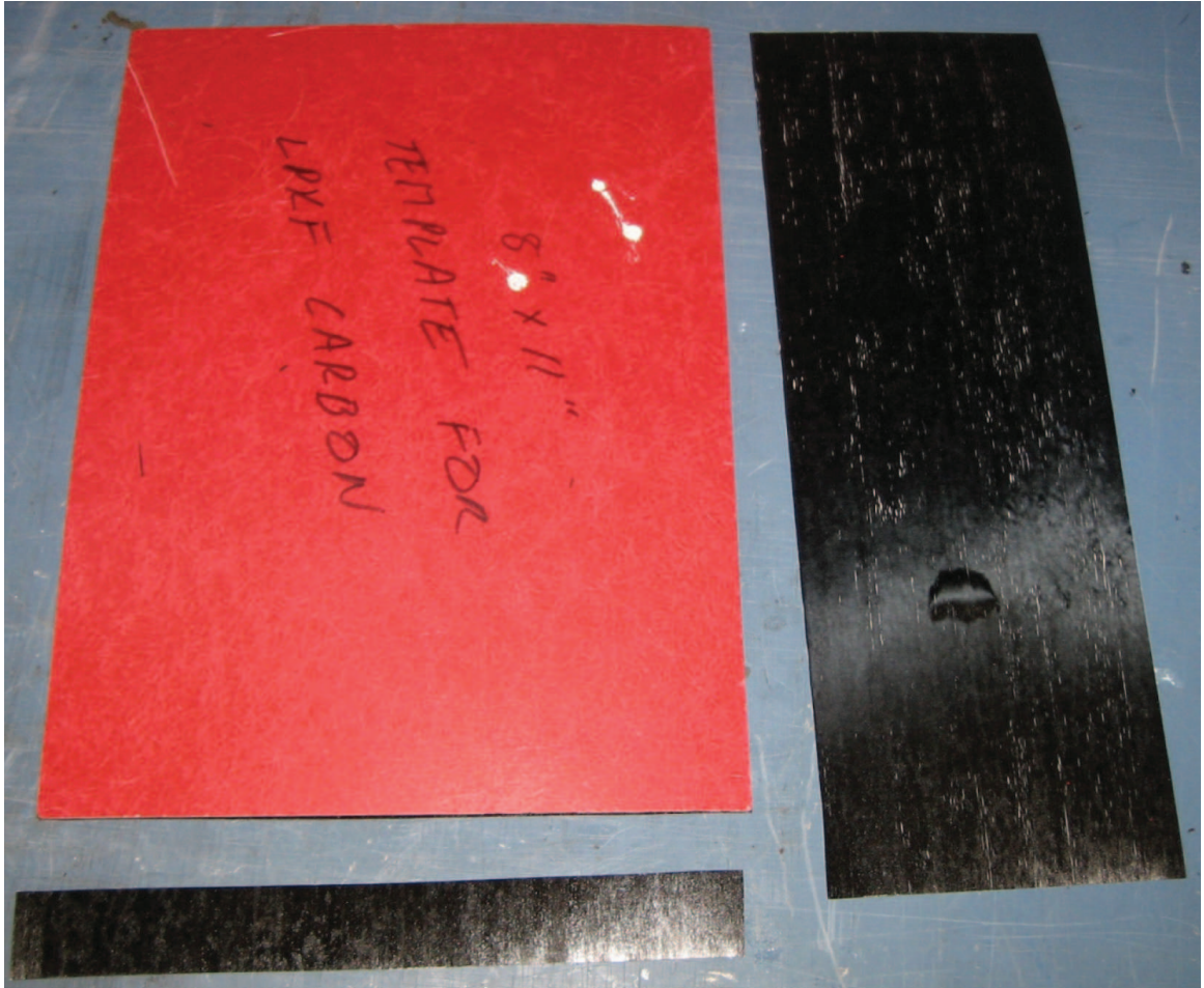
Figure B.1: Carbon cut from square sheet in the “0” direction utilizing the carbon cutting template.
