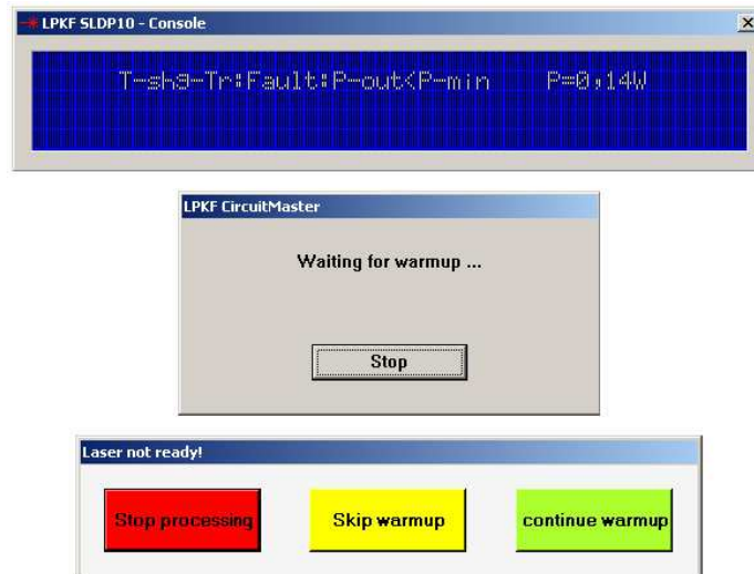
Figure B.2: The three pop-ups that are shown and used during the ProtoLaser U warmup procedure.
