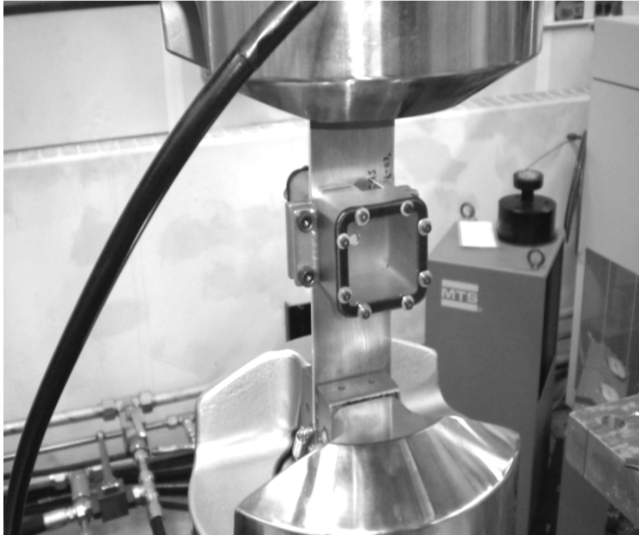
Figure 3.7: A chamber with salt water installed on the specimen.
