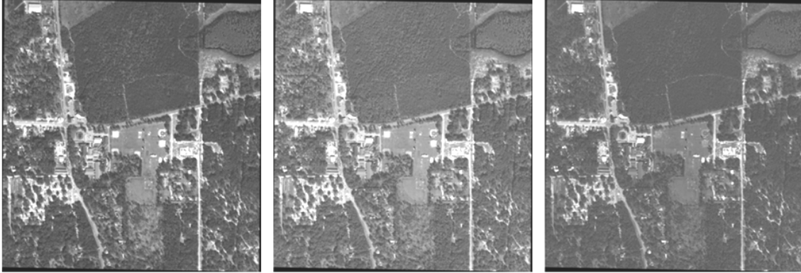
Figure 20. Left to right: The red, green, and blue texture maps generated by transforming the FLDOT RGB imagery to lidar space using the registration results.
