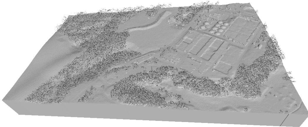
Figure 17. The resulting geometry produced from the synthetic “original” images written in obj format and rendered using Meshlab.
