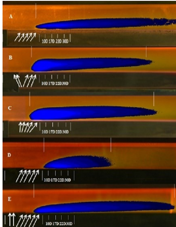
Figure 0.53: Flame Visualization, \phi = 1.3 , M = 2.0 , A-Five Row, B-Two Row Upstream, C-Roll Forward, D-Swirler, E – Cross Flow
