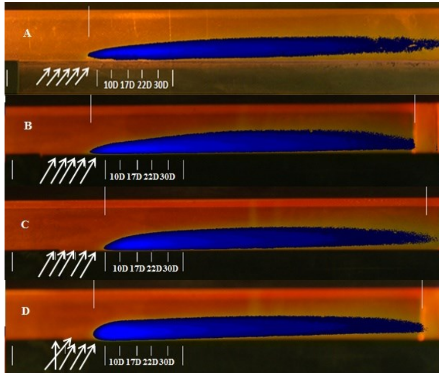
Figure 0.40: Flame Visualization, \phi = 1.3 , M = 2.0 , A-Five Row, B-Five Row Slot, C-Five Row Trench, D-Backwards Facing Step
