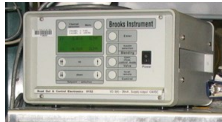
Figure 0.31: Brooks, 0-10 SLPM, mass flow controller for film cooling air/N 2
