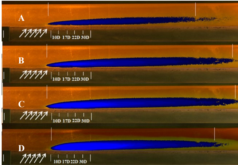
Figure 0.37: Five Row Flame Visualization, Equivalence Ratio Sweep, A – \phi = 1.1 , B – \phi = 1.175 , C – \phi = 1.3 D – \phi = 1.4 , M = 2.0
