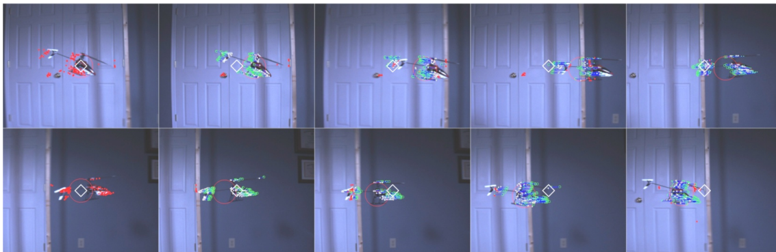
Figure 5.12: A sequence of frames, approximately 0.24 seconds apart for one period, of a swinging test subject with the center of the image identified by a white diamond, previous points shown as green rectangles, \mathbf{g}_{i-1} , current optical flow points as white, closed circles, \mathbf{g}_i , estimated points as green, open circles, \hat{\mathbf{g}}_i , and removed outliers shown as red, closed circles.
