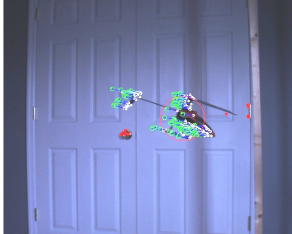
Figure 5.10: A moving test subject captured by a static camera with previous points shown as green rectangles, \mathbf{g}_{i-1} , current optical flow points as white, closed circles, \mathbf{g}_i , estimated points as green, open circles, \hat{\mathbf{g}}_i , and removed outliers shown as red, closed circles.
