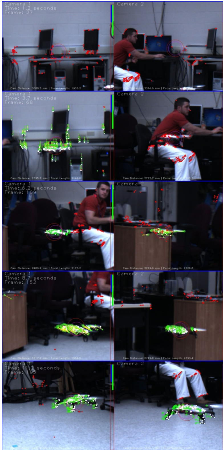
Figure 6.13: X-axis testing of the quadcopter’s 3D position using Vicon and “two-camera, PTZ system”.
