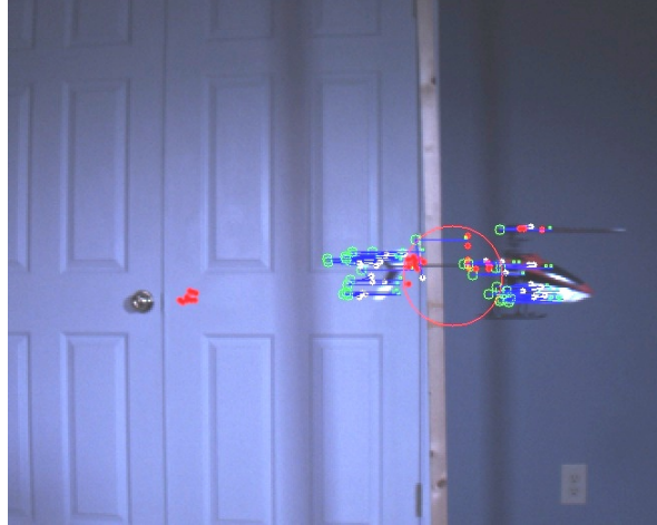
Figure 5.11: A moving test subject captured by a moving camera with previous points shown as green rectangles, \mathbf{g}_{i-1} , current optical flow points as white, closed circles, \mathbf{g}_i , estimated points as green, open circles, \hat{\mathbf{g}}_i , and removed outliers shown as red, closed circles.
