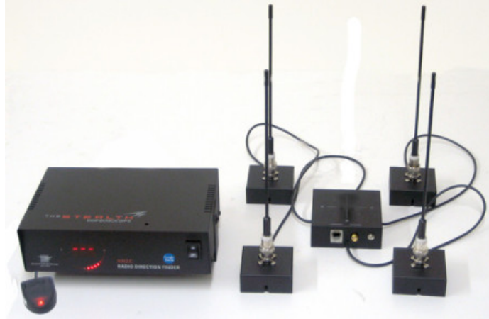
Figure 3.2: KN2C Doppler Direction Finding System [37]
