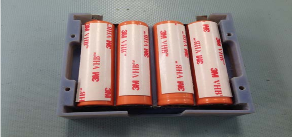
Figure 27: Thermal Adhesive on Battery Cells
