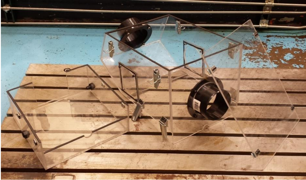
Figure 44. The new thermal cooling box disassembled for installation around the engine.
