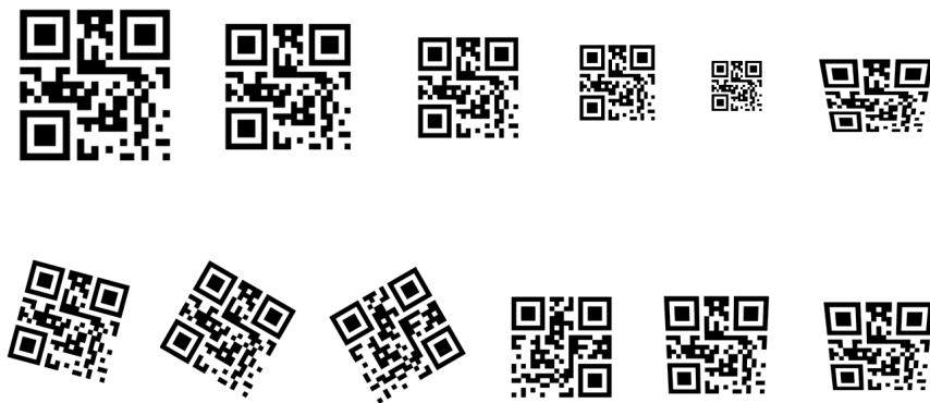
Figure 21. This image set was created to validate the properties of the SURF algorithm, namely scale and rotation invariance. A QR code is used as the feature set in the images and is rotated, scaled, and skewed to simulated multiple view angles for detection.
