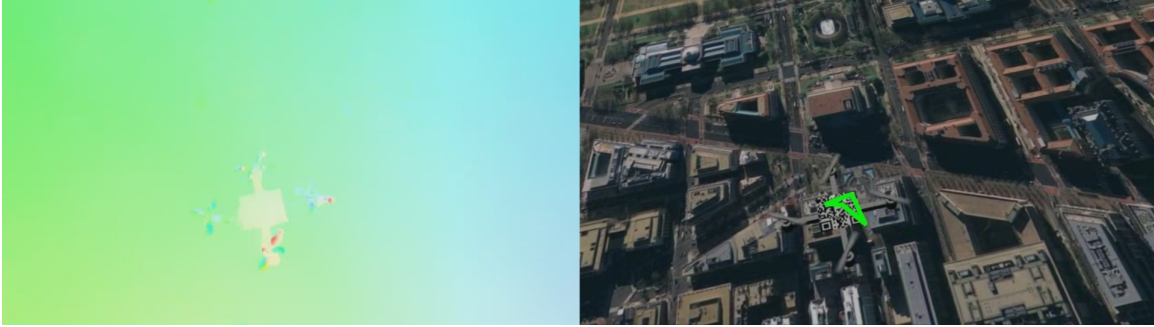
Figure 2. The current point of the approach scenario shows the homography estimation algorithm failing because of distance, but the optical flow algorithm has a solid lock on the target.
