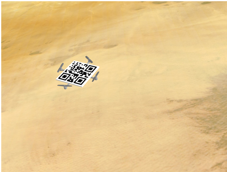
Figure 24. This scenario image shows the QR code painted on the airborne landing platform that will be approached by a UAV with a mounted camera. In the final meter of approach towards the platform, the homography estimation resulting from Discrete SURF matches will be determined.
