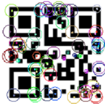
Figure 26. Features detected by the FPGA detector are sent back to the PC through a serial connection and plotted in MATLAB. Interior dots show feature location, whereas circle diameter indicates scale.
