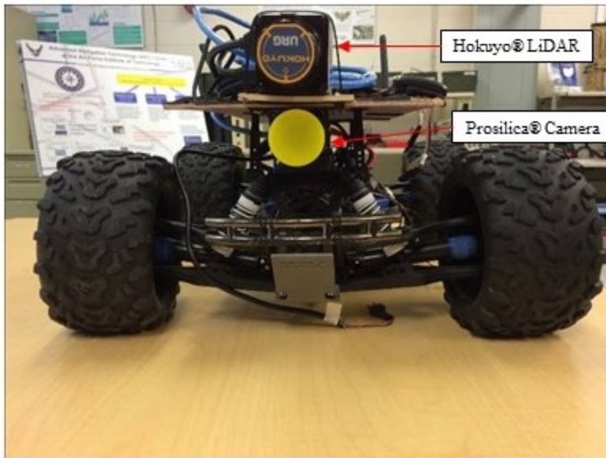
Figure 13. LiDAR and camera attached to platform (prior to 3D printed brackets).
