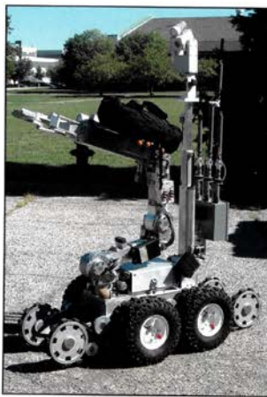
The new bracket exceeded expectations during testing, saving EOD technicians 60 to 90 seconds when changing sensors. (U.S. Air Force photo/Maria Meeks/Released)
