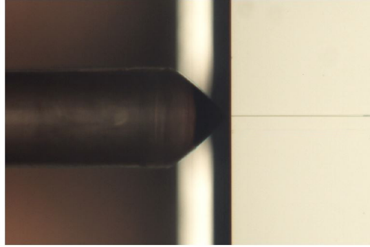
Figure 29. A microscope image of the alignment of the lensed fiber to the Si wire waveguide.
