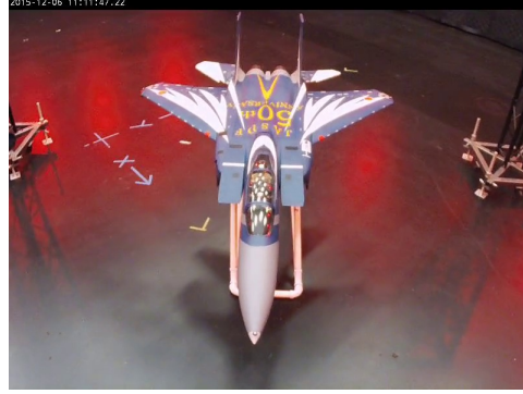
Figure 22. Raw image captured by the imaging system. A sample image, i_{t,x} output by the image capture stage. It is associated with a particular camera, C_x , and a particular time, t .
