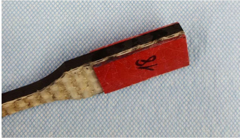
Figure 6. Unitized composite specimen with fiberglass tabs
