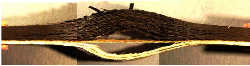
Figure 39. Stitched optical micrographs of MS3 0/90° specimen T5-2 following failure in tension at room temperature and load removal. From Wilkinson [3]
