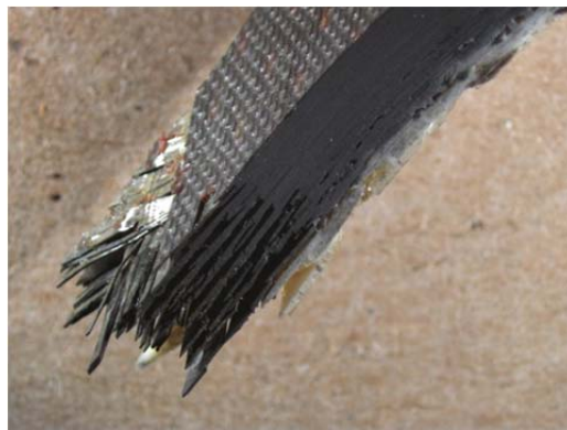
Figure 46. Optical micrograph of specimen T8-1 viewed from an angle after failure in tension-tension fatigue at 76 MPa.
