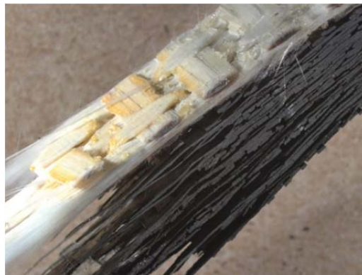
Figure 42. Optical micrograph of specimen T7-4 viewed from an angle after failure under tension-tension fatigue at 430 MPa.
