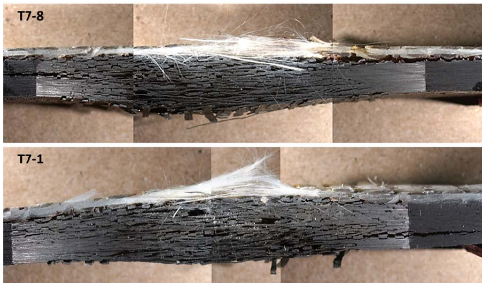
Figure 38. Stitched optical micrographs of the MS4 0/90° specimens T7-8 and T7-1 after failure in tension at elevated temperature.
