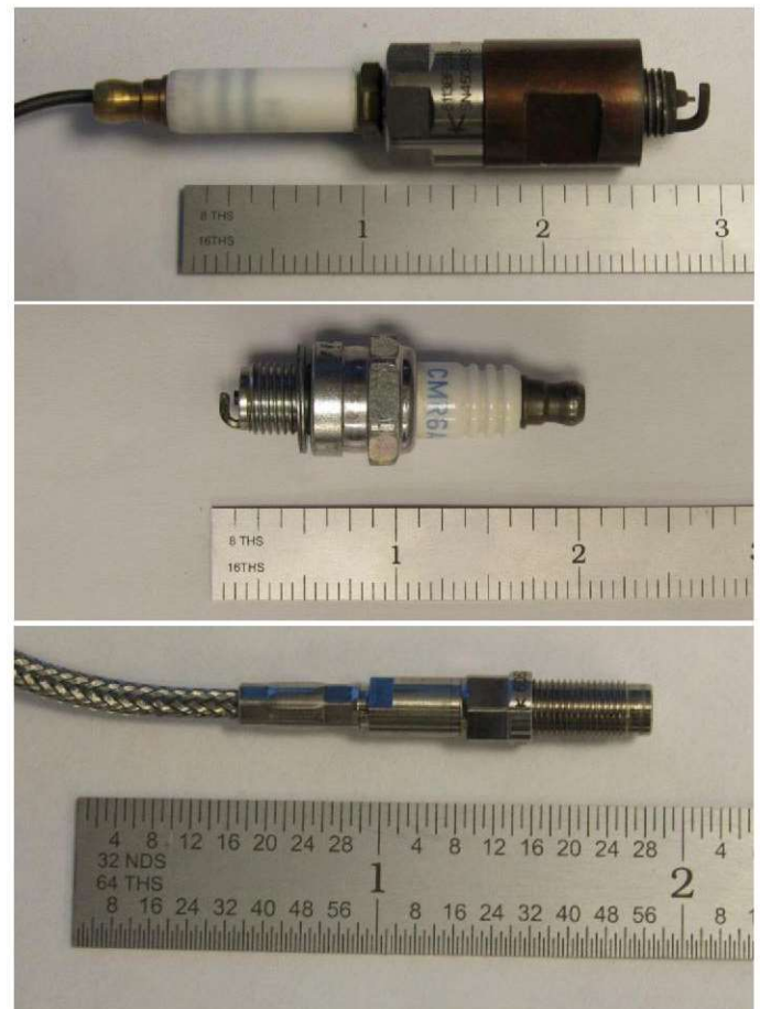
Figure 5. Top: Custom Kistler Measuring spark plug with copper spacer washer installed. Middle: Stock CM-6 spark plug. Bottom: Kistler Flush Mount Pressure Transducer
