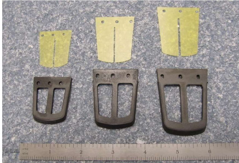
Figure 168: Reeds and reed carriers for the 3W-28i (left), 3W-55i (middle) and 3W-85Xi (right) engines.
