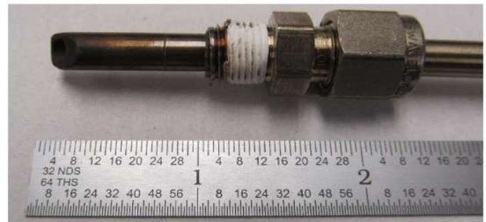
Figure 3: Sampling probe used on the SERB.
