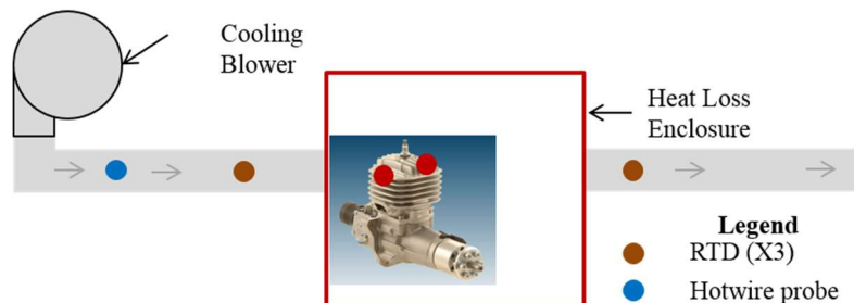
Figure 54: Schematic of SERB cooling air system components.
