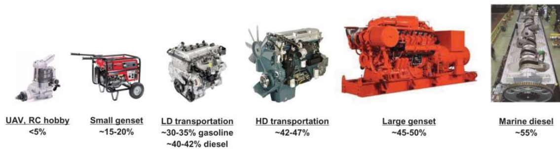
Figure 15: Typical fuel conversion efficiencies of various sizes of engines, reprinted with permission from Edwards et al. [100].
