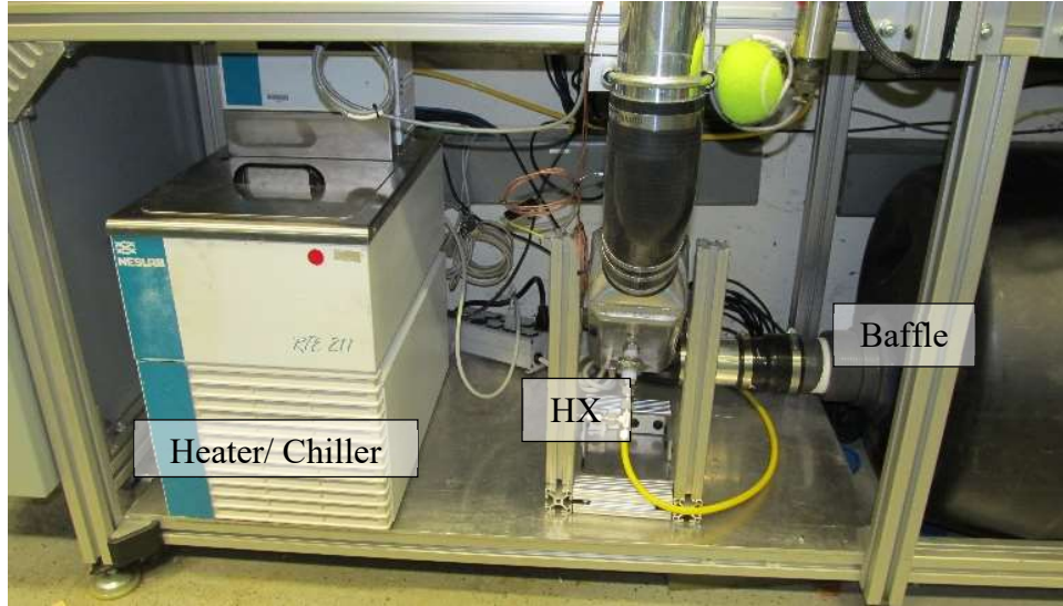
Figure 51: Photograph of SERB showing the intake air system.
