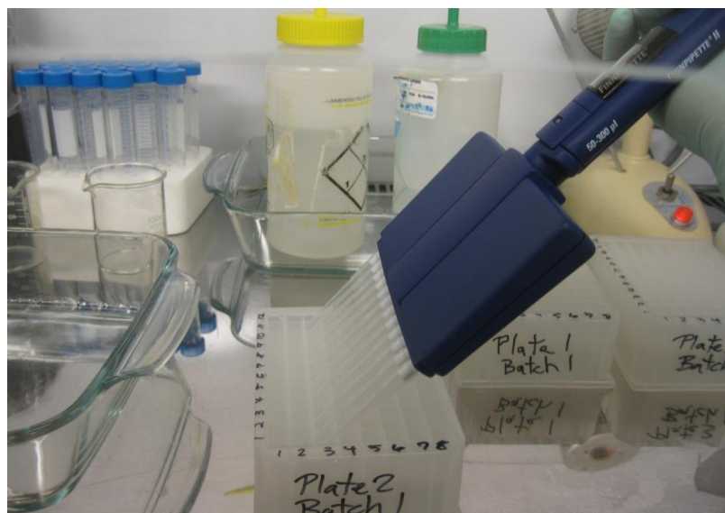
Figure 21. Twelve-tip pipette used in microdilutions
