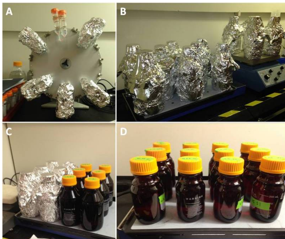
Figure B 8. Experimental reactor bottle configurations. Figure A displays the tumbler with 50 mL vials in triplicates. Figure B illustrates the 1 L bottles covered with aluminum foil on stir plates. Figure C shows the 500 mL reactor bottles, and Figure D displays the 250 mL amber bottles selected as the final standard configuration
