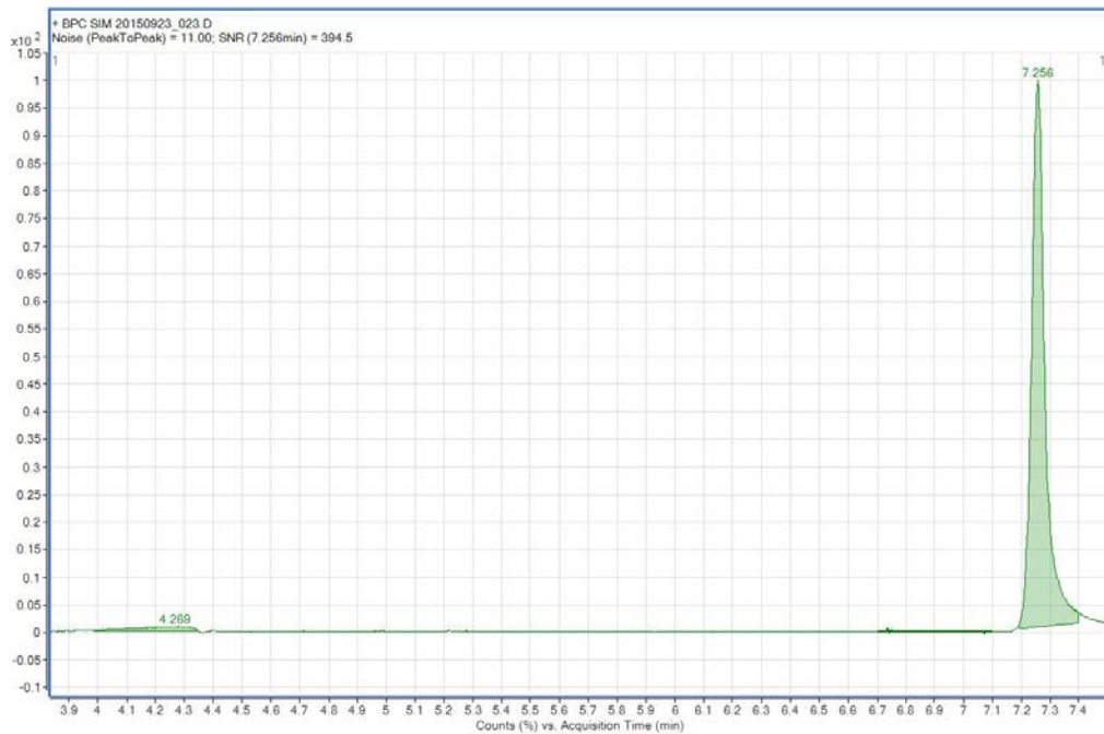
Figure B 27. DNT peak is on the far right of the figure and occurs at 7.256 minutes with 14172.11 area counts. Observed for C_0 of the \sim 1.5 \text{ mg L}^{-1} control collected during the CNT-Foam isotherm experiment
