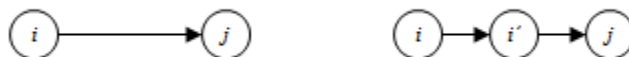
Figure 23. Arc (i, j) is split and proxy node i' takes its place
