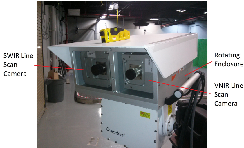
Figure 3.3. A sensor similar to the AisaDUAL hyperspectral sensor. A SWIR line scan camera (left) and a VNIR line scan camera (right) are contained in the rotating enclosure.
