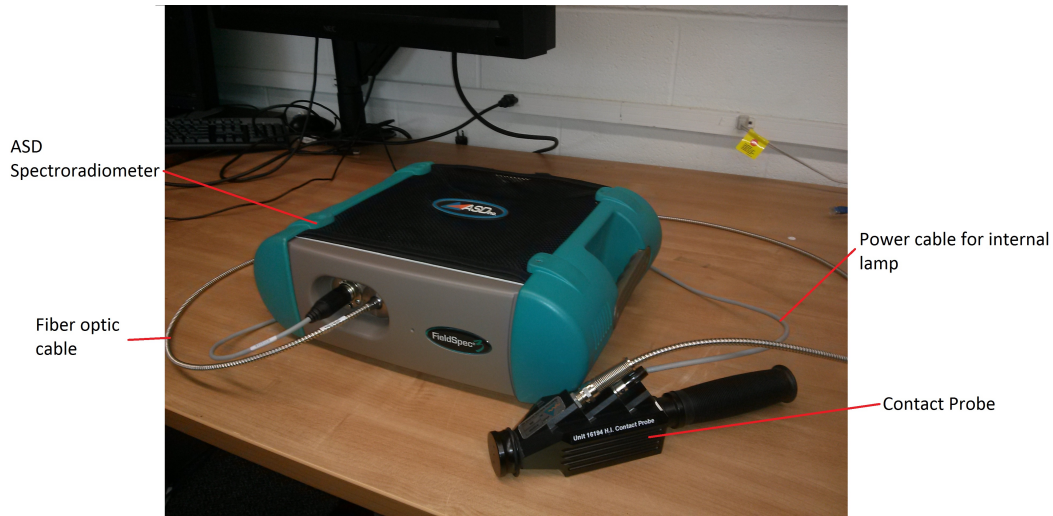
Figure 3.2. The ASD Fieldspec ® 3 spectroradiometer and contact probe. The power cable for the halogen light source and the fiber optic cable are shown connected from the spectroradiometer to the contact probe.
