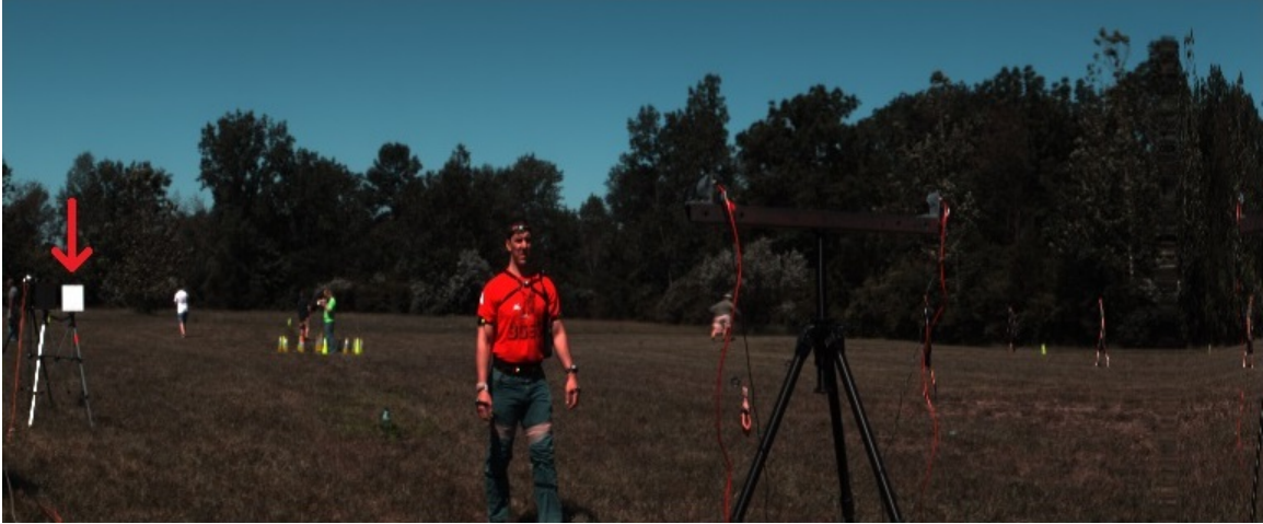
Figure 3.4. A color representation of the hyperspectral image used to determine noise variance. The Spectralon white reflectance panel (indicated by a red arrow) is on the left.
