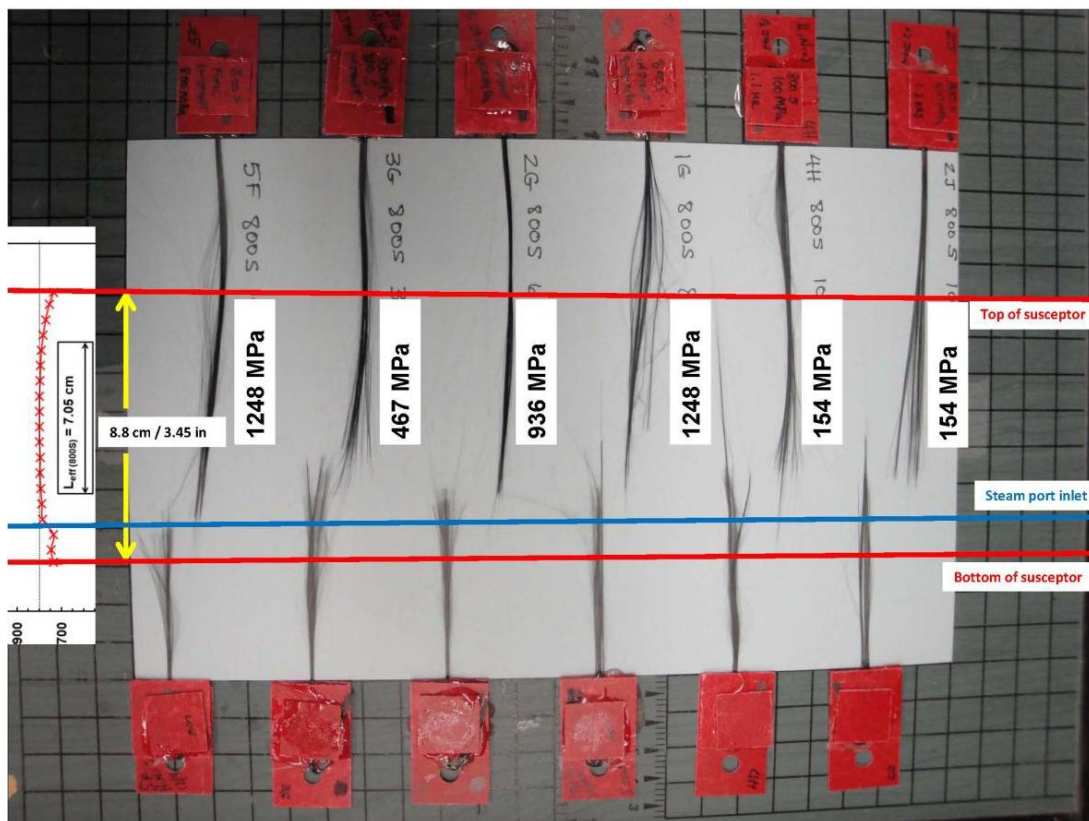
Figure 25: Effect of steam impinging on fiber tows upon entry into the test chamber; reproduced from Steffens [32]
