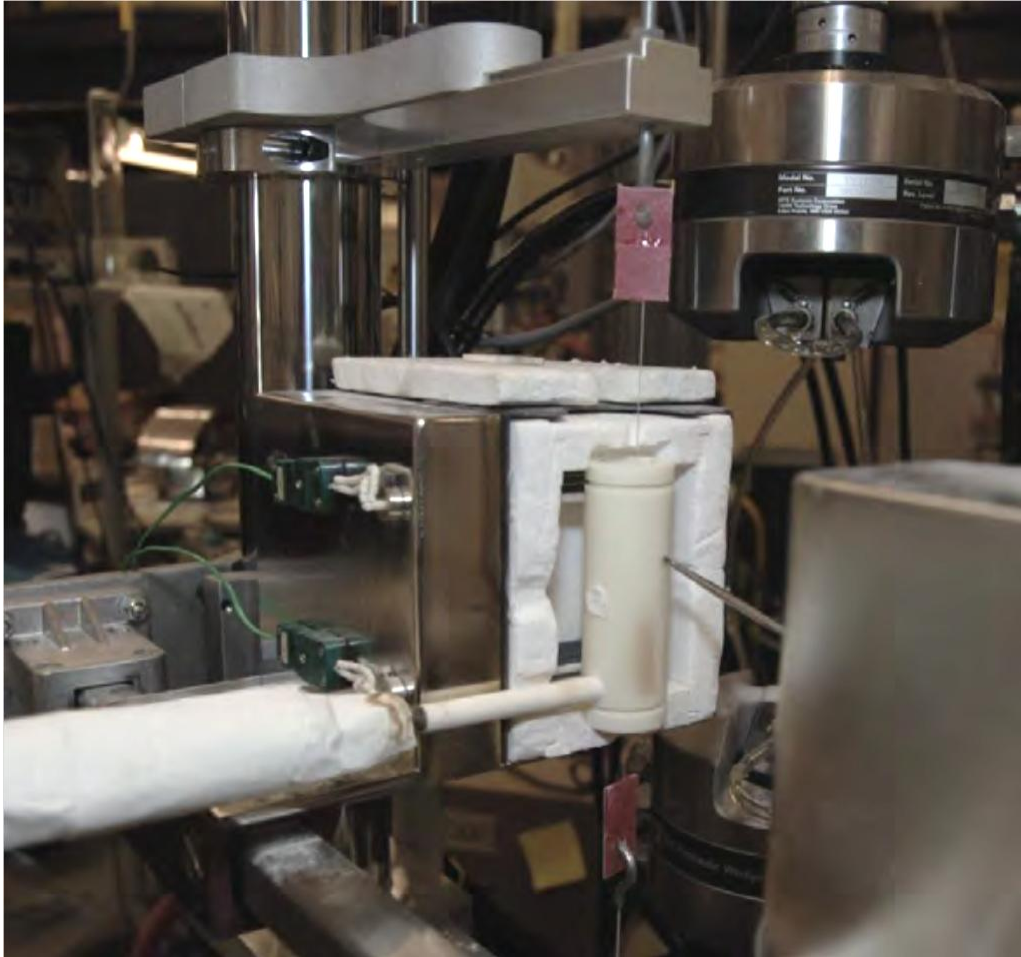
Figure 21: Alumina susceptor and feeding tube assembled in one half of the furnace, along with fiber tow specimen mounted and running through the alumina susceptor; reproduced from Armani [15]
