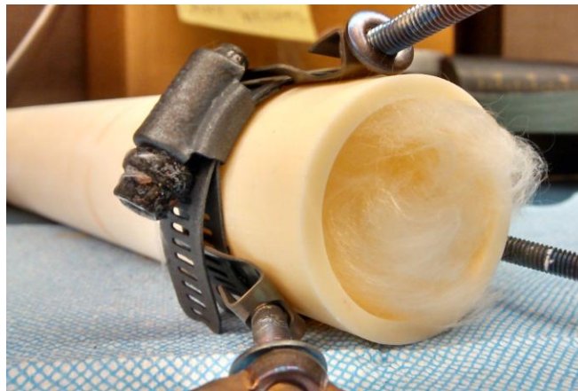
Figure 29: Silica wool placed inside the heating tube to achieve saturation of heated steam with silicic acid
