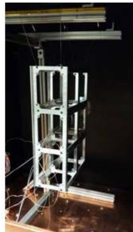
(b) The Chassis including Heaters in TVAC
