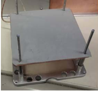
(a) Thermal Conductive Pad Used between the Heat Dissipater Bottom Face and the Circuit Board
