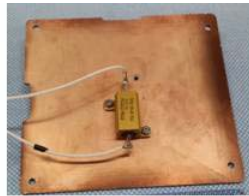
(a) SHCB (The Circuit Board with a Vishay 10W Capacity Resistor)
