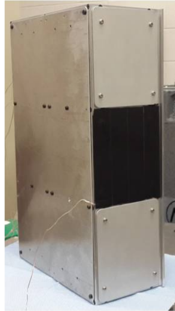
(b) The Sample CubeSat with Black Photo Tape Covered 1U Radiator (ET-G)
