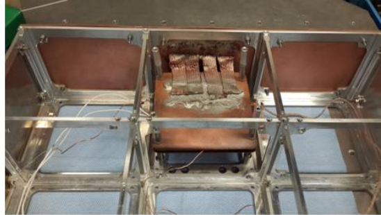
(a) 3U Size Radiator Connected to the Heat Dissipater Using Soldered Thermal Straps
