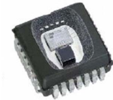
Figure 1: BOSCH high-g accelerometer for vehicle airbag system from 1990s [5].
