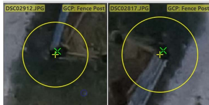
Figure 14: Position deviations between computed location from 2-D match points (Green cross) and input GCP coordinates (Yellow cross) on the same feature point in two images.
