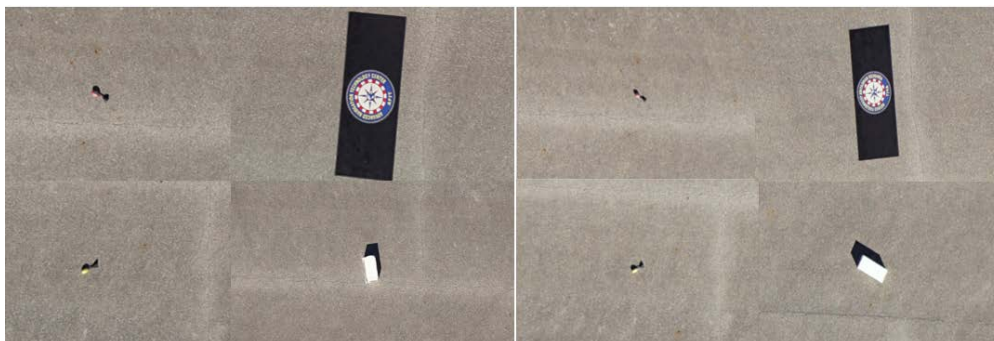
Figure 23: Object identification of orthomosaic by 25 meters altitude flight(left) and 50 meters flight (right).
