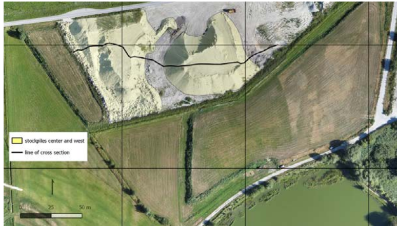
Figure 7: Top view of surveyed stockpile (Site A) with line of cross section [21].
