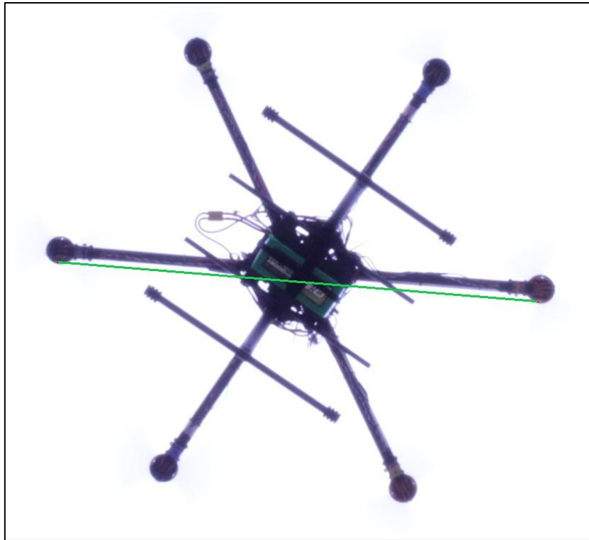
Figure 16. Yaw Angle Measurement Example
