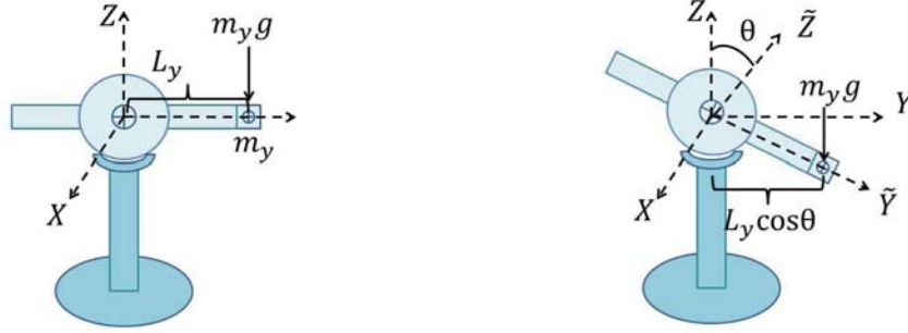
(a) Satellite Simulator Imbalance Y-Axis (b) Torque Due to Imbalance in Y-Axis
