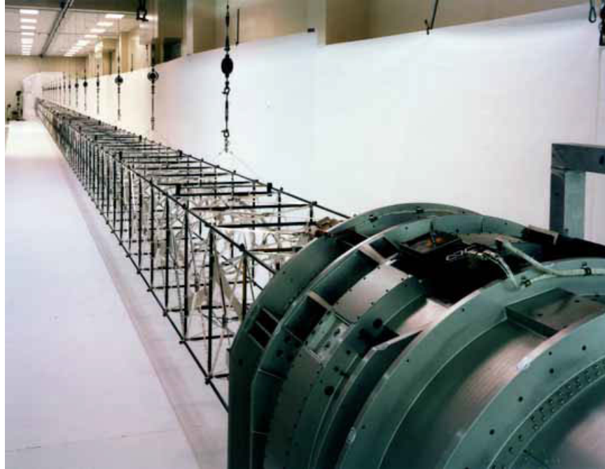
Figure 5. ADAM deployed from canister in laboratory environment with gravity off-loading [3].
