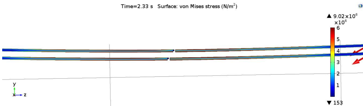
Figure 51. Uncontrolled deployment simulation stress at 2.33 seconds. (Cropped)
