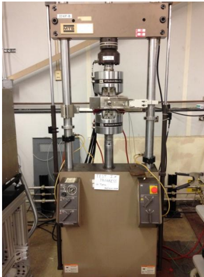
Figure 10: 810 MTS Machine Setup
