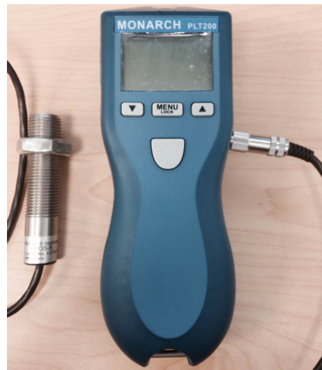
Figure 49. The Monarch PLT200 Optical Tachometer
