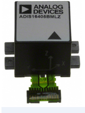
Figure 21. ADIS Model 16405 IMU
