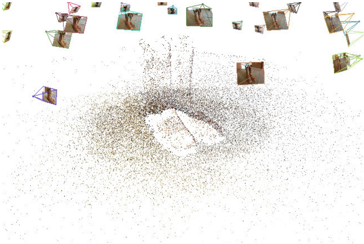
Figure 5. The output of the sparse reconstruction step, performed in the VisualSFM program
