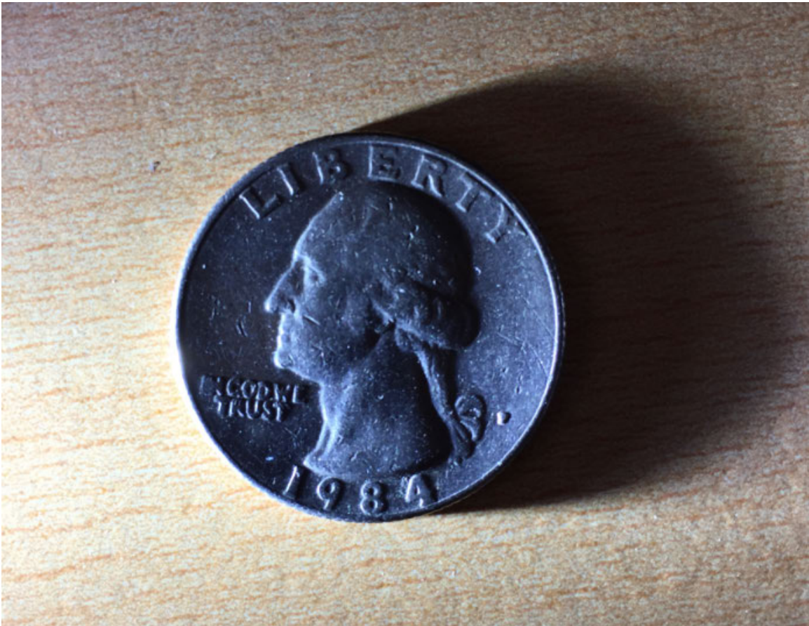
Figure 1. A quarter with strong light source from the left; edges on the left are bright white, but edges on the right are dark, causing potential confusion to automated analysis programs
