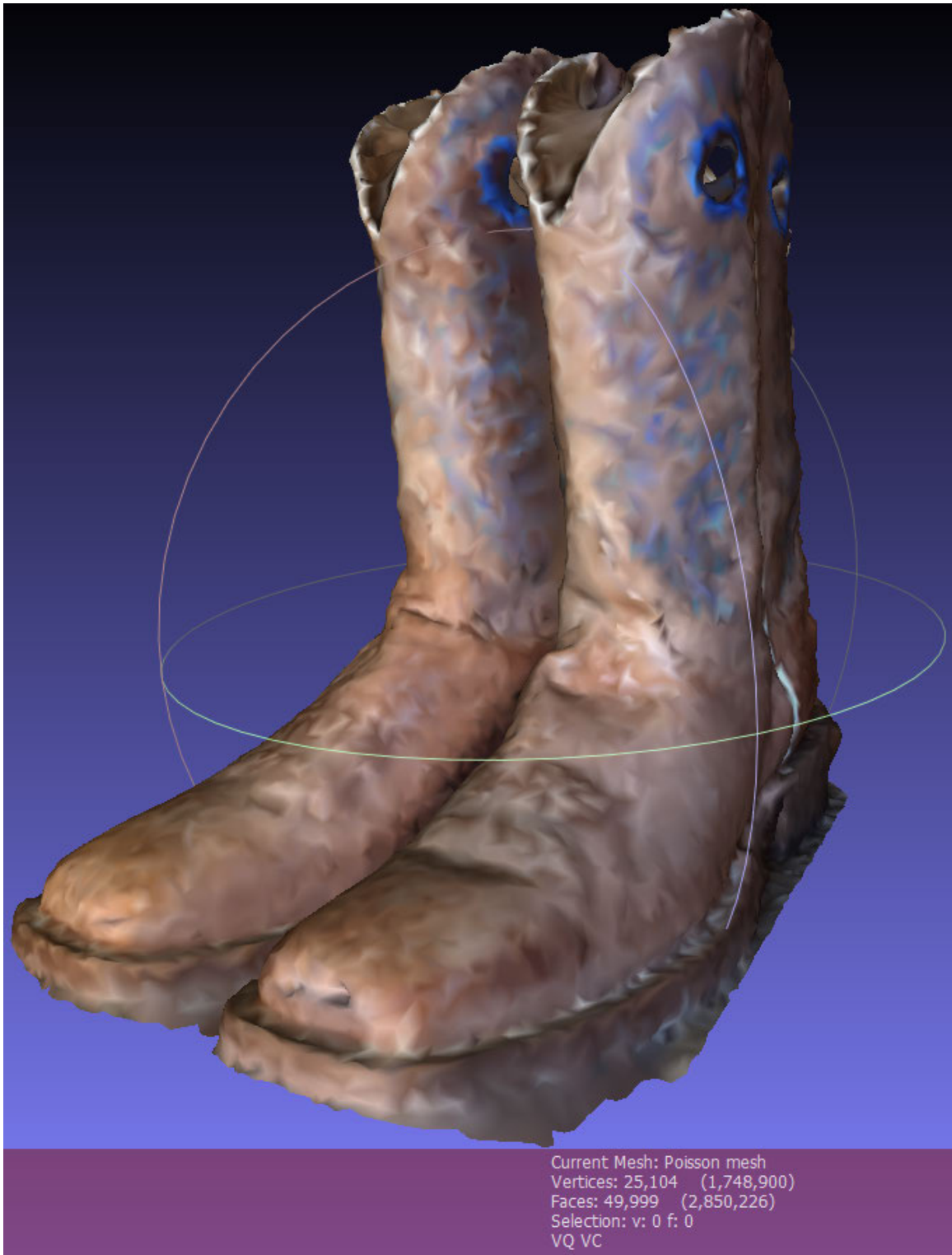
Figure 9. The result of decimating the model to reduce the number of vertices
