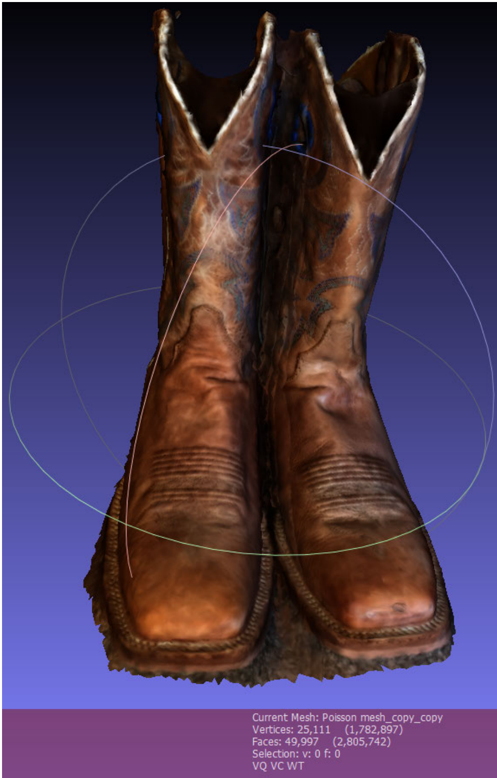
Figure 10. A final, textured model created by a SfM pipeline with some manual processing
