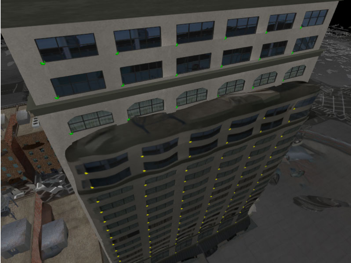
Figure 19. Visualization of geopoints; green dots represent truth data, and yellow dots represent reconstruction data. The spatial difference between each corresponding pair quantifies the distortion of the reconstruction.
