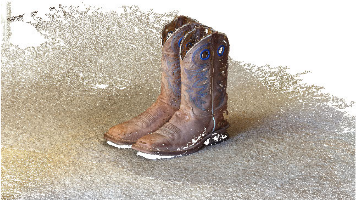
Figure 6. The output of the dense reconstruction step, performed in the VisualSFM program
