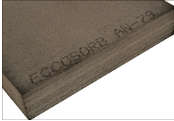
Figure 7. Section of ECCOSORB ® AN-79 foam block
