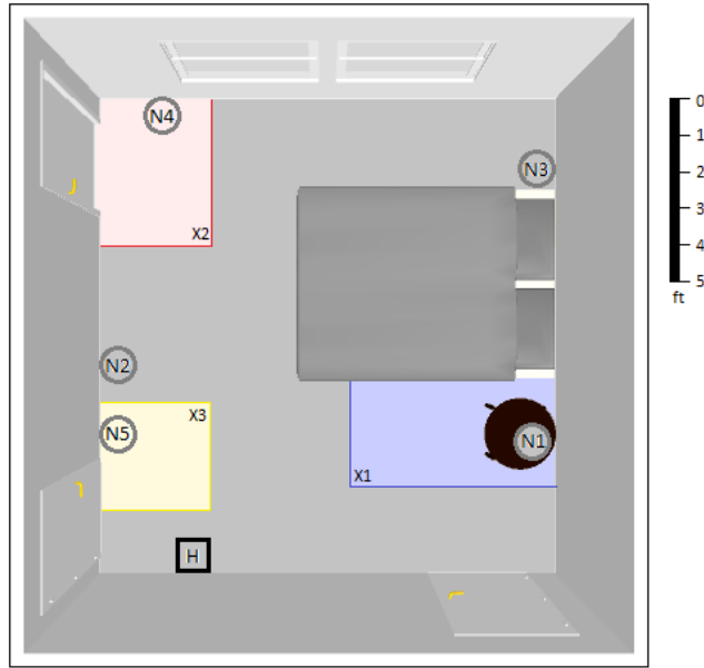
Figure 34. Diagram of Room C showing regions (X#) for context-based localization
