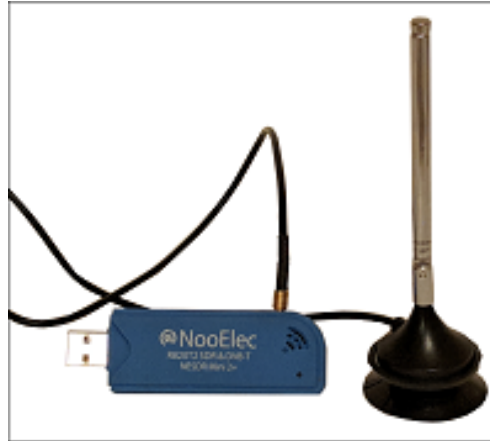
Figure 6. NooElec receiver and antenna used for data collection
