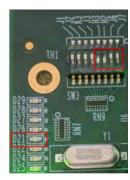
Figure 47. Various dip switch states showing the correct function of an OR gate.
