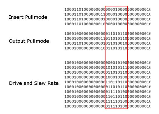
Figure 38. Comparison of bitstreams generated for pin T16.
