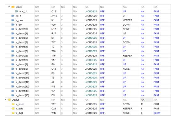
Figure 28. Pins and their configuration options used in the bitstream parser test.
