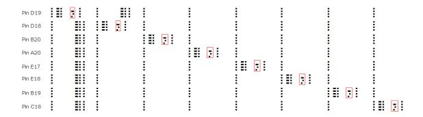
Figure 29. Selection of bitstreams related to the pullmode configuration of group 1 input pins with 1's replaced with black space and 0's replaced with white space.
