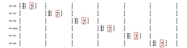
Figure 33. Selection of bitstreams related to the pullmode configuration of group 4 pins with 1's replaced with black space and 0's replaced with white space.
