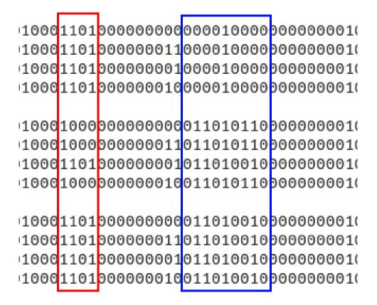
Figure 43. Portions of bitstreams related to indices controlling input, output, and bidirectional options for pin D17.
