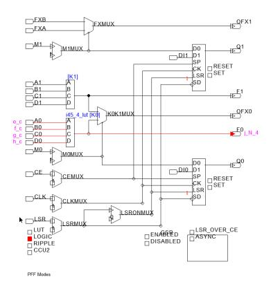
Figure 2. Example configurable logic block.
