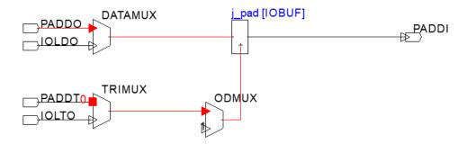
Figure 4. Example input-output block.
