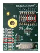
Figure 48. Various dip switch states showing the correct function of an AND gate after a bitstream modification attack.
