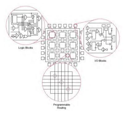
Figure 1. FPGA Architecture showing CLBs, IOBs, and Interconnects [20].
