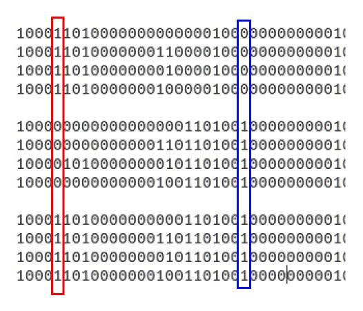
Figure 42. Portions of bitstreams related to indices controlling input, output, and bidirectional options for pin D19.
