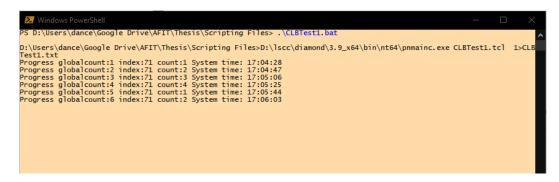
Figure 11. TCL script running generating bitstream files for analysis.
