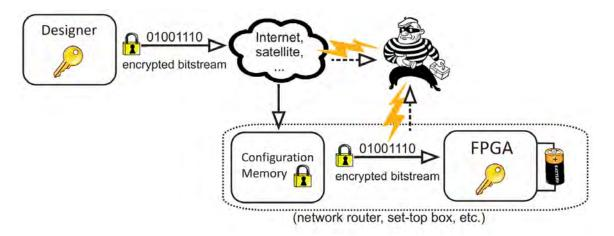
Figure 7. FPGA receiving encrypted bitstream from designer [17].
