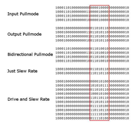
Figure 37. Comparison of bitstreams generated for pin D17.
