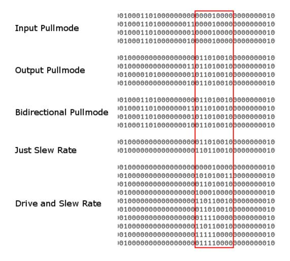
Figure 36. Comparison of bitstreams generated for pin D19.
