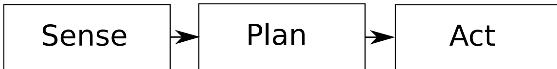
Figure 1. The flow of information through the deliberative paradigm. Information is first sensed. Then a plan is created based on an environmental representation created from sensed data. Finally, the plan is carried out in the act phase.
