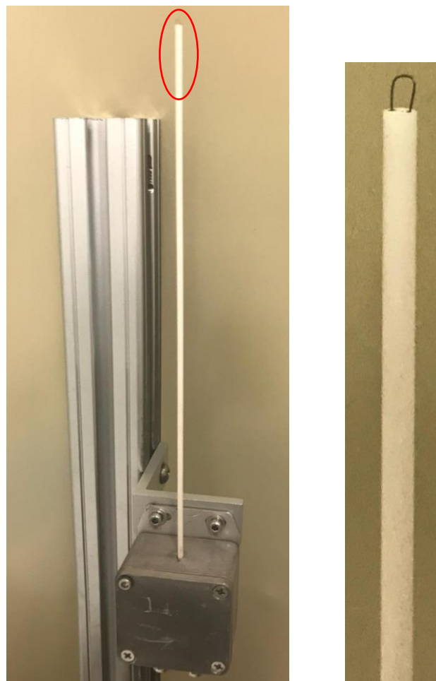
Figure 3.14: Emissive Probe. Right image is detail of area circled in red on left.
