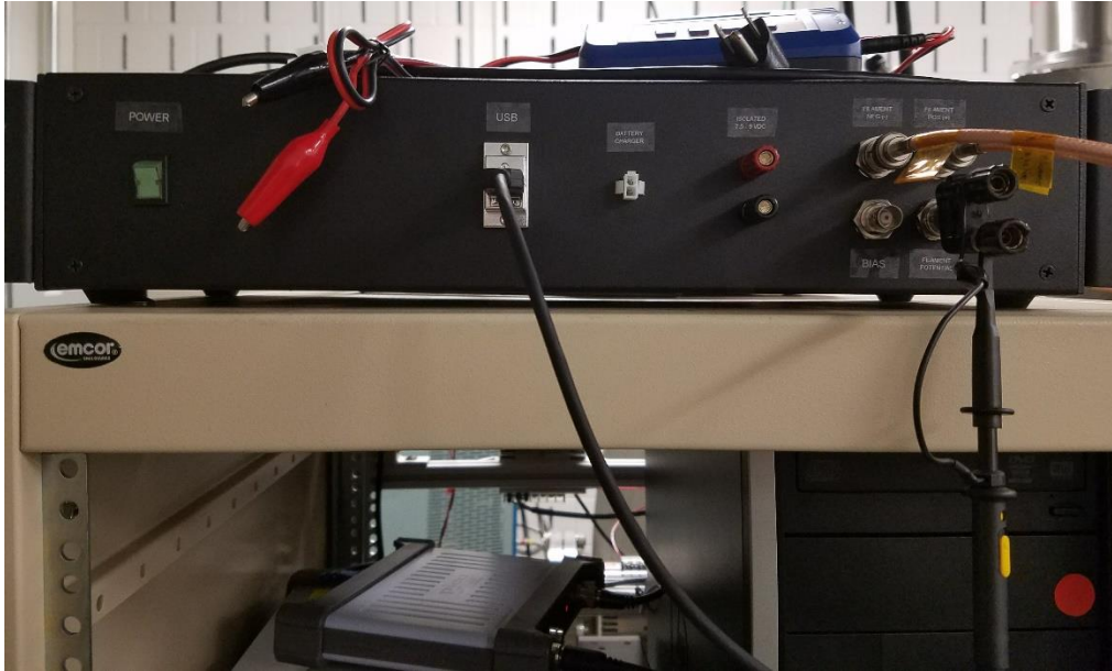
Figure 3.15: Emissive Probe Control Box, PicoScope DAQ, and Recording PC
