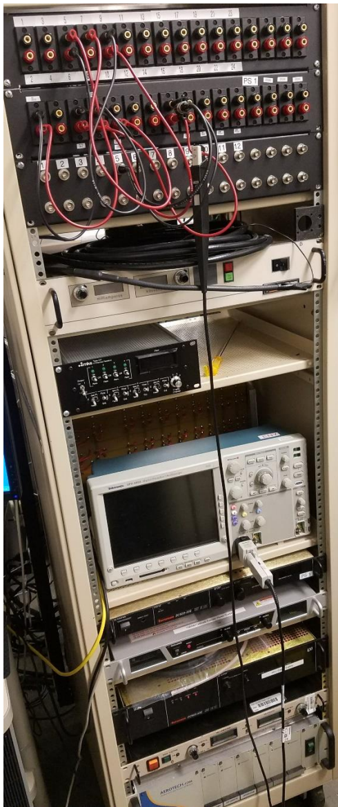
Figure 3.5: Power Supply and Mass Flow Control Rack
