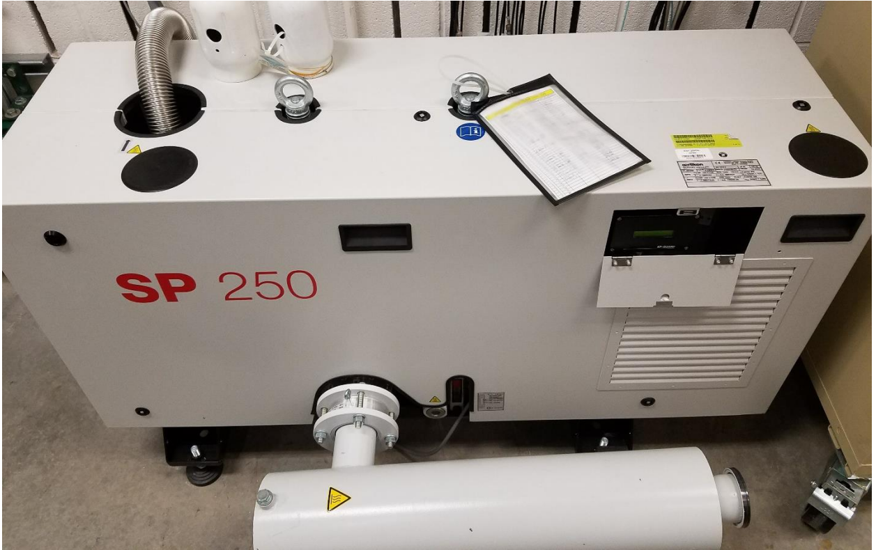
Figure 3.9: Oerlikon/Leybold SP 250 Roughing Pump
