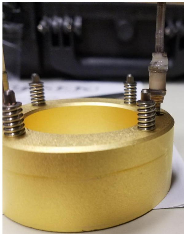
Figure 3.22: Repair Attempt 1: taken during epoxy cure time
