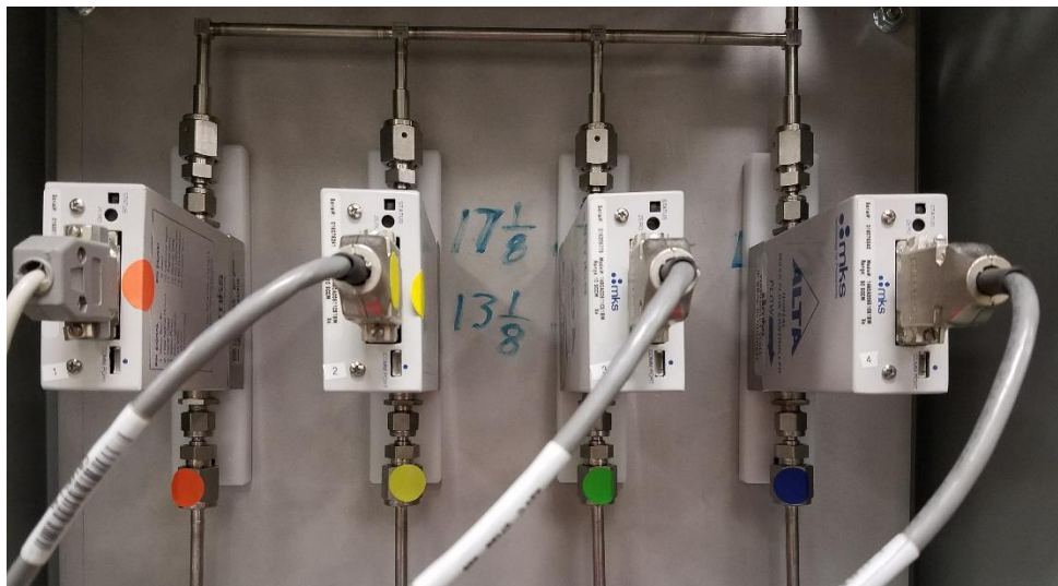
Figure 3.6: Mass Flow Controllers
