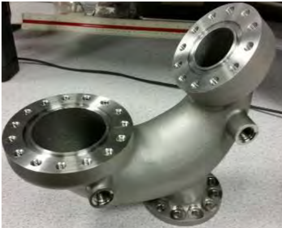
Figure 5. Additively manufactured fuel mixer pipe [14]
