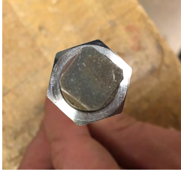
Figure 35. Blocked opening before sanding
