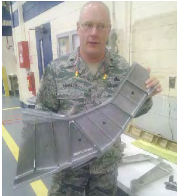
Figure 6. Subtractively manufactured C-5 end fitting [18]
