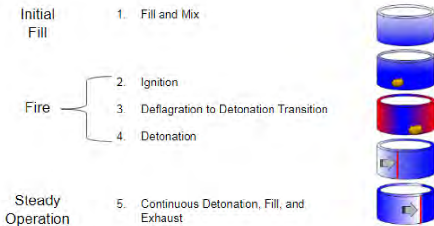
Figure 2. RDE Detonation Process [21]
