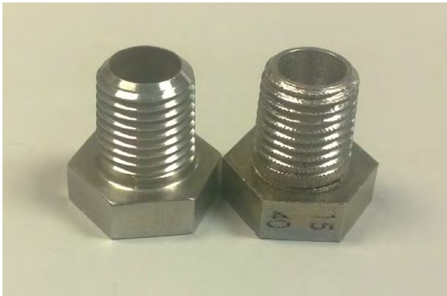
Figure 7. Machined micro nozzle (left) and DMLS Nozzle (right) [24]
