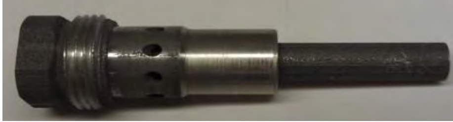
Figure 4. Additively manufactured single element injector [14]
