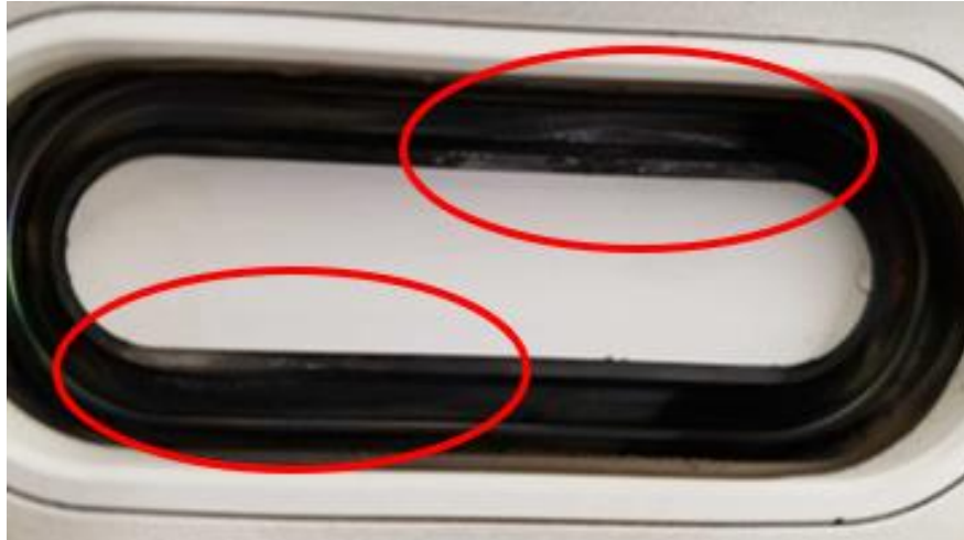
Figure 41: Visual Erosion on Channel
