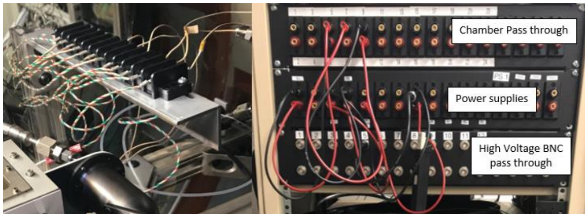
Figure 9: Chamber patch panels interior (left), exterior (right)
