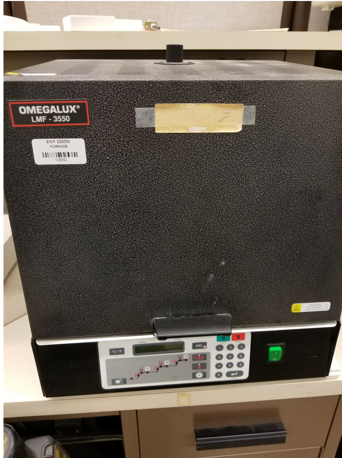
Figure 3.16: Omegalux oven used for curing the conductive ink on the adhesive substrate
