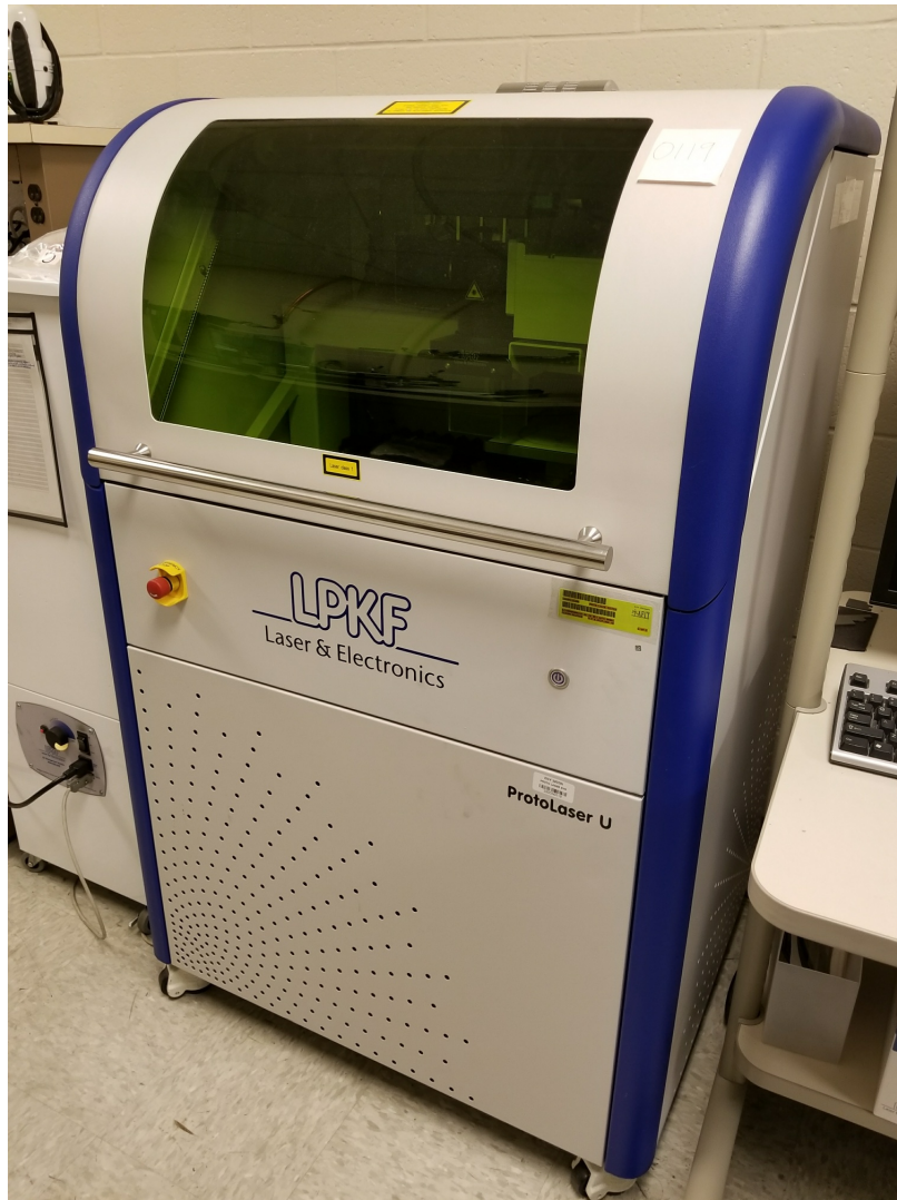
Figure 3.2: LPKF UV-laser used for cutting out substrate and thin film materials for specimen creation
