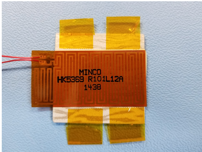
Figure 3.12: Etched foil heater with Kapton® mounting tabs
