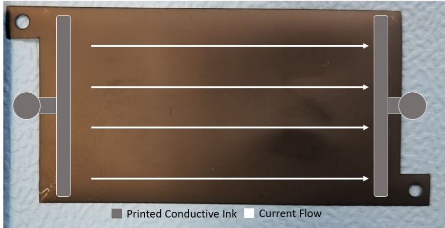
Figure 3.18: RS100 specimen intended current flow design
