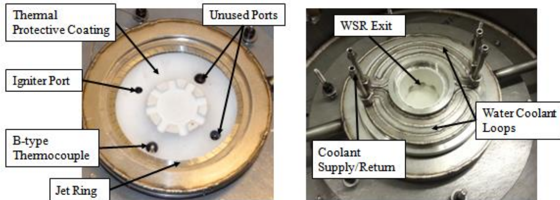
Figure 3-3: Lower toroid and jet ring (left), upper toroid (right)
