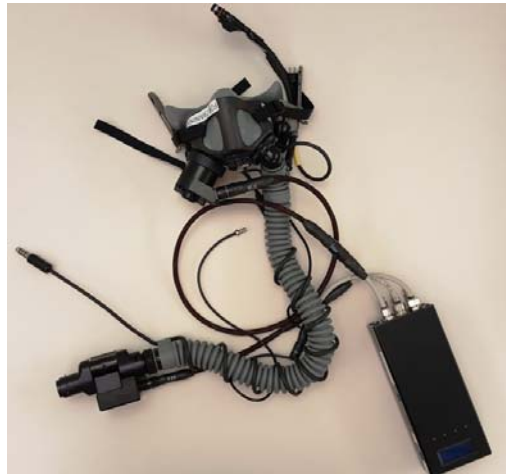
Figure 11: AMPSS 2.5 - Modification to MBU-20/P Flight Mask
