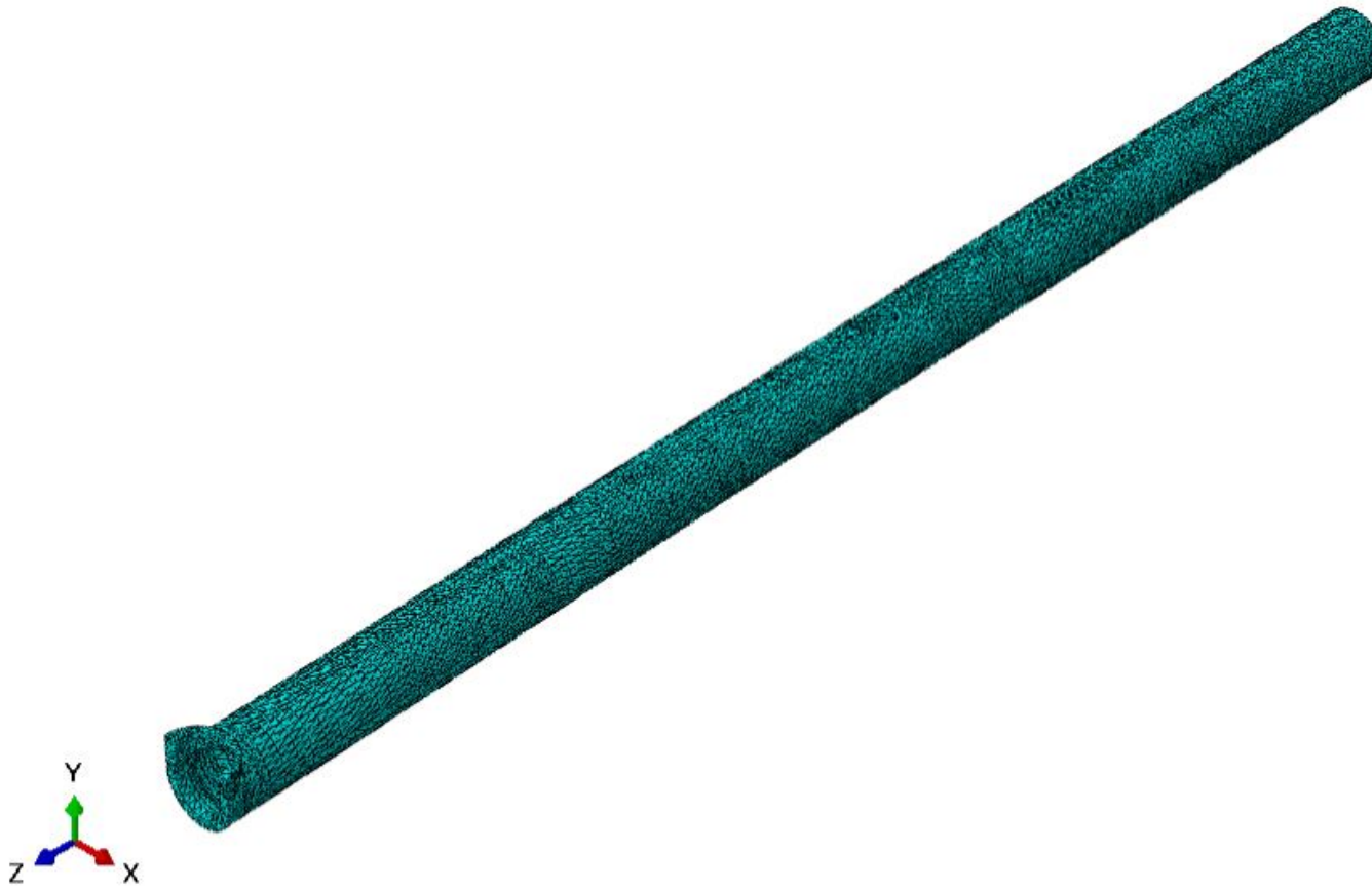
Figure 3.11. Meshed air evacuation system 1
