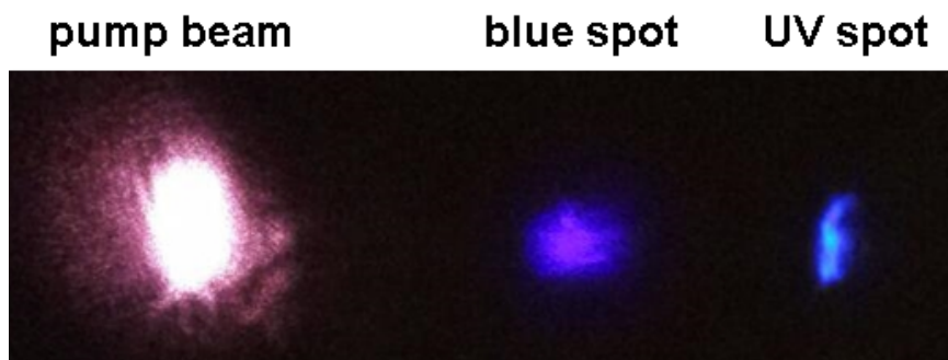
Figure 5.4: Beam emissions for the Cs cell in the forward direction at 1.5 m.
