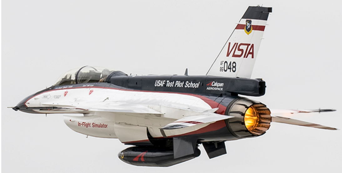
Figure 2. The US Air Force Test Pilot School NF-16D Variable stability In-flight Simulator Test Aircraft (VISTA) [47]
