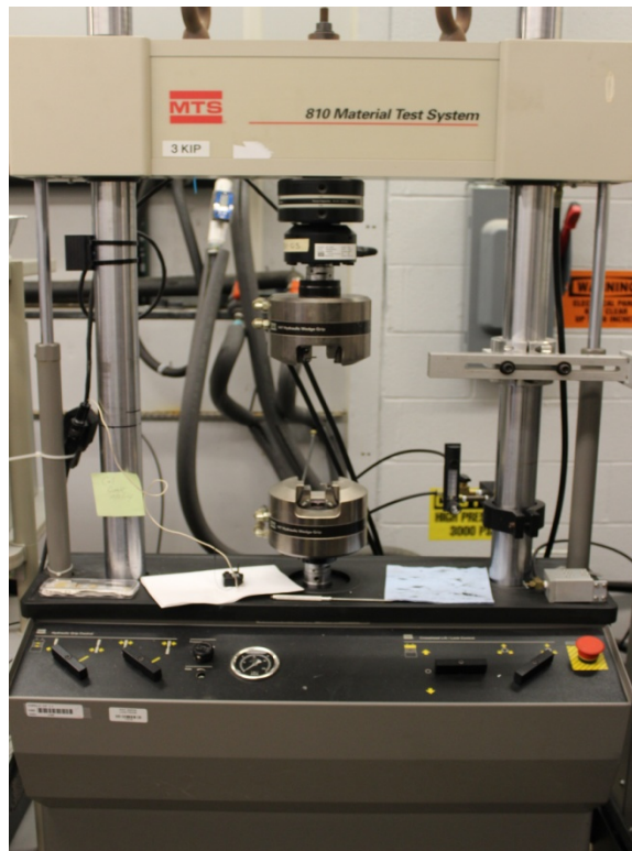
Figure 4 – MTS 810 Material Test System utilized for uniaxial tensile testing
