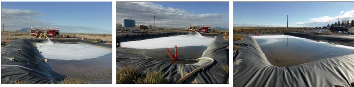
Figure 12. INL Field Site, Water Security Test Bed. Lagoon contains 8,000 gallons of water and is spiked with 5 gallons of AFFF.
