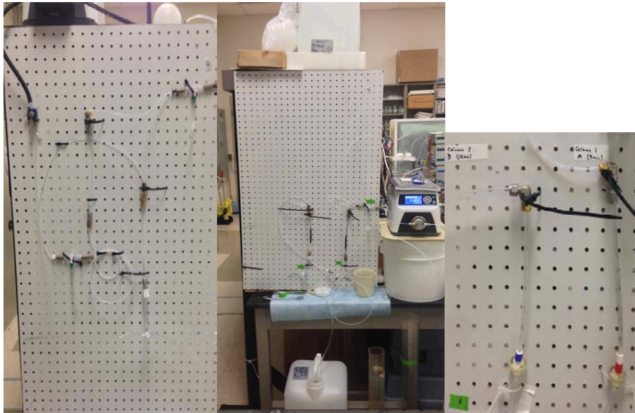
Figure 11. RSSCT Experimental design. RSSCT columns (no GAC); Influent, pump, columns and effluent; Detail of columns with nylon filter (No GAC or glass wool). (Left to right)
