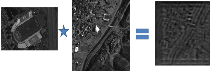
Figure 2.9: Aircraft image correlated with satellite image. The images must be rotated in the same direction and images must be of equal scale. Note the white peak in the resulting image denoting the region of maximum correlation (ie. the location where the images match).
