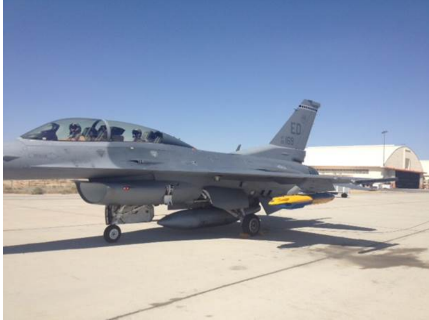
Figure 3.1: The RASCAL pod (yellow and blue pod under the wing) containing the MAMI-II payload is shown mounted on an F-16.
