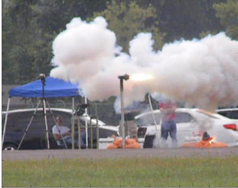
Figure 16. Picture of the Smoky SAM during combustion. The Smoky SAM was held in this fixed position for the duration of the test. The observed plume was approximately 2 - 3 ft long and burned for 5 seconds.
