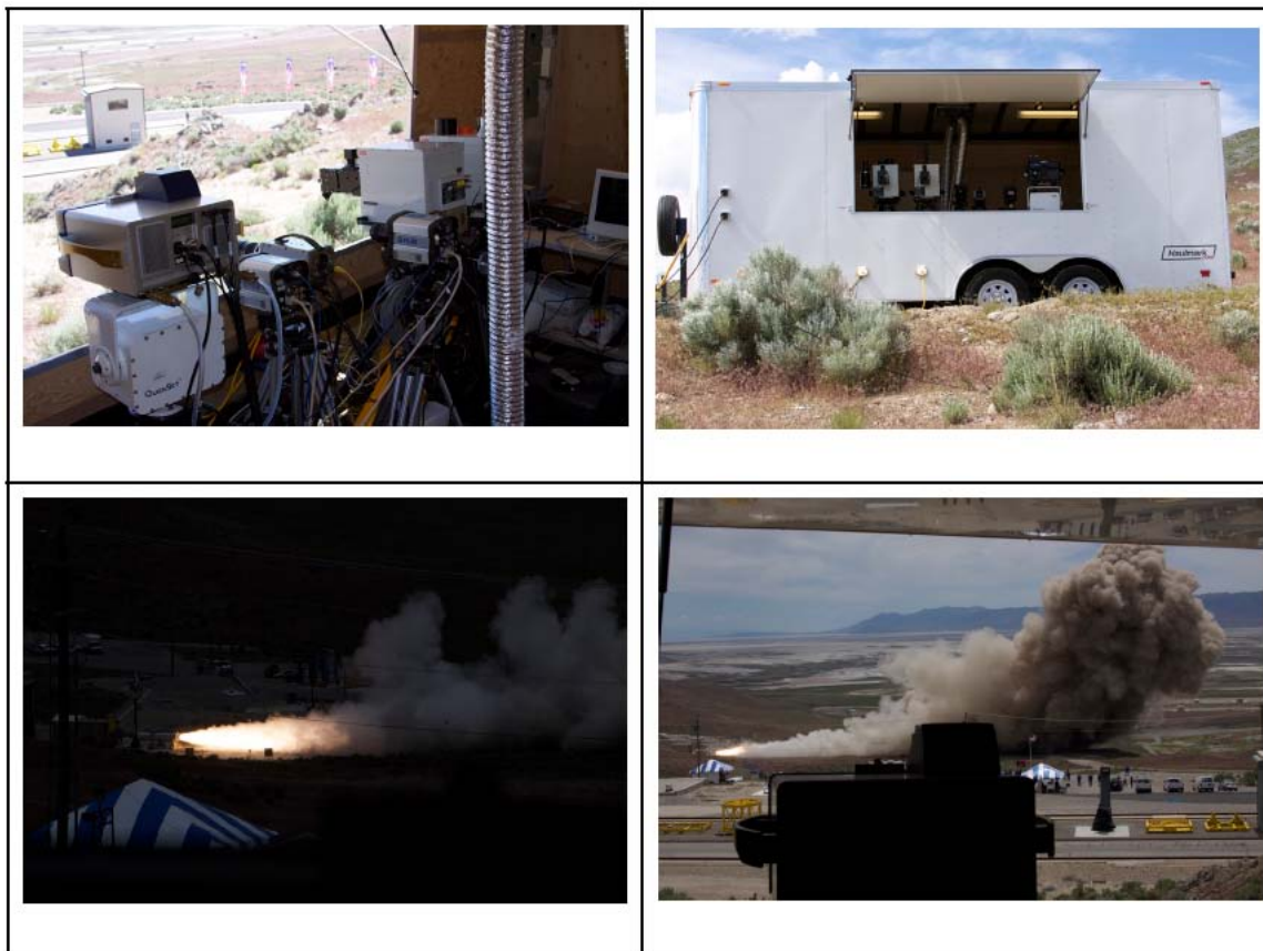
Figure 20. Pictures of the static solid rocket motor test. Top row: pictures of the instrument suite setup in the AFIT remote sensing trailer. Bottom row: pictures of the solid rocket motor and emission plume during ignition.
