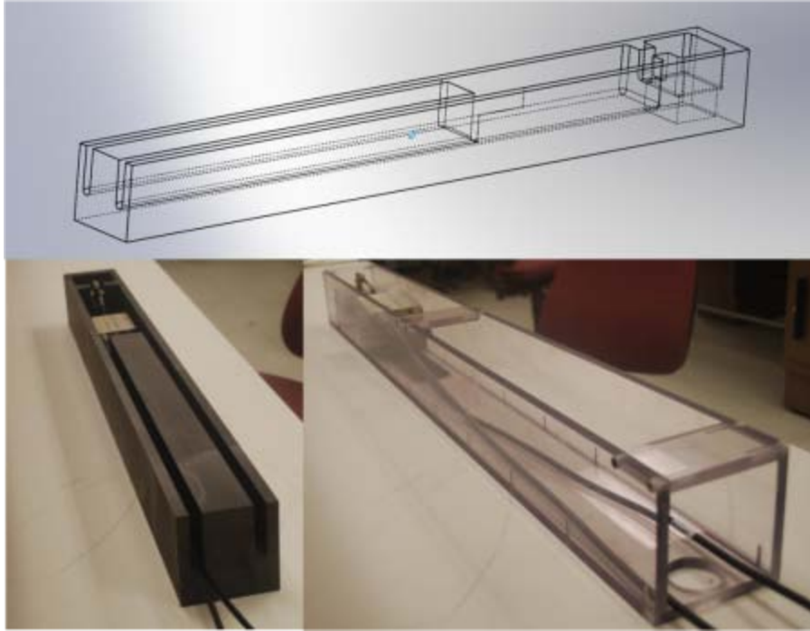
Figure 28. The graphite and Lexan versions of the mock stringer or “sled” created for use in this experiment are shown above as well as the design submitted to the AFIT model and fabrication shop. The dimensions of the sleds are slightly smaller than the standard graphite stringers used to construct the AFIT graphite pile, as well as the OSURR thermal column and sub-critical reactor. These dimensions allow for modularity of experimental set-up and ease of insertion of the detector into the neutron environment.
