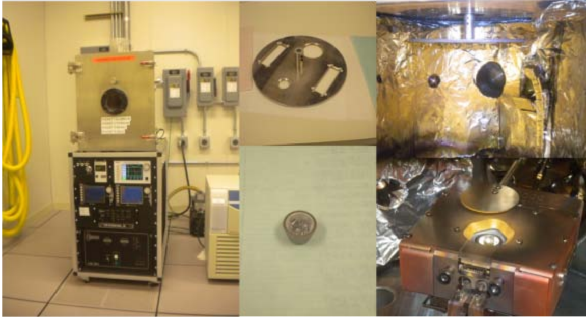
Figure 21. The Electron Beam Evaporator in the AFIT Clean Room used to deposit contacts on the samples is shown in the left of the figure. Samples were fastened to the the mask and loaded into the spindle (top middle), which was then secured in the evaporator chamber (top right). The hearth in the floor of the chamber (bottom right) can accommodate up to five crucibles (bottom middle) loaded with a target metal.
