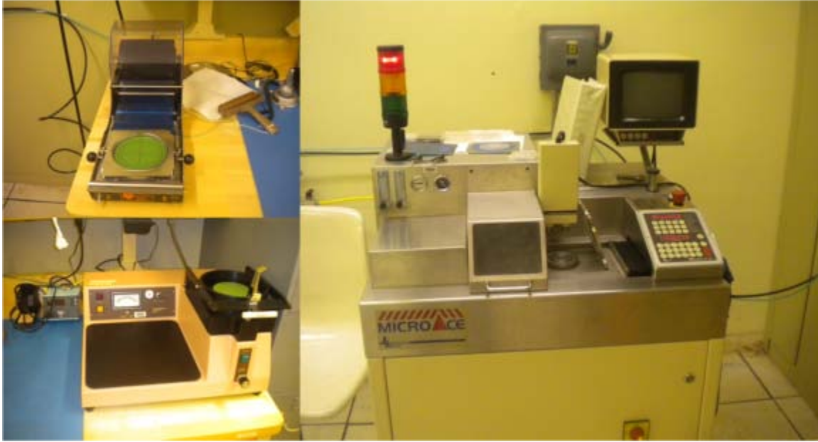
Figure 20. The uncut samples were placed on the Micro Automation Model 140 mounting station (top left) and pressed with high tack tape. The frame and tape with the sample attached was then heated on the Die Matrix Expander (bottom left). Once the tape had heated sufficiently to securely adhere the sample, the frame was loaded onto the Micro Ace saw (right).
