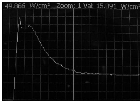
Figure 16. Image of the power meter showing rise, overshoot, fall, and steady state
