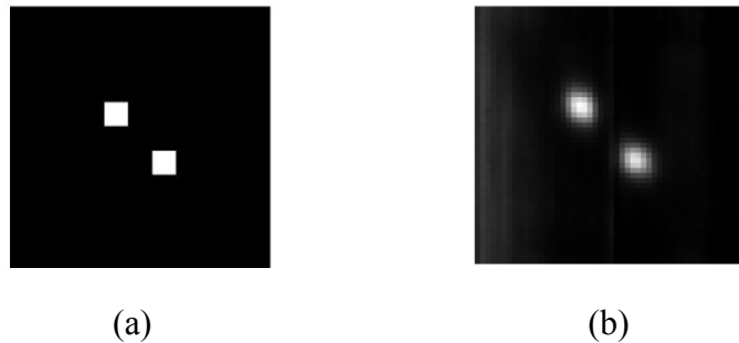
Figure 2. Object of interest (a) and its indirect image (b) created without either the camera or the light source having line-of-sight to the object
