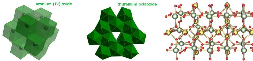
Figure 1. Crystalline structure of \text{UO}_2 , \text{U}_3\text{O}_8 , and \text{UO}_3 . [20]
