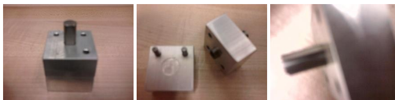
Figure A- 1: Gold Stamp. The gold stamp consists of two machined aluminum blocks and a serrated carbide plunger. The sample is placed gold side up between the two aluminum blocks and the serrated tip is used to impress lines onto the gold surface. Subsequently turning the upper block 90 degrees and impressing a second set of lines will create a grid.
